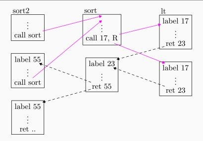
The CFI security policy dictates that software execution must follow a CFG path determined ahead of time.
